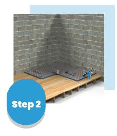
Screw the MARMOX BOARDS to the timber floor tightly by using MARMOX washers along with chipboard screws at a rate of 12 per sheet. Seal wet areas joints and cover all washers with MS Polymer.
