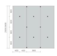
Positioning of dowels for full surface bonding of boards with 900 mm width starting with 10 mm thickness.
