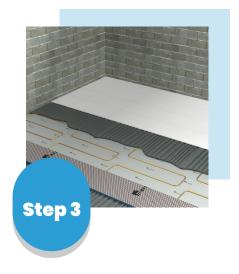
Install the underfloor heating system according to the manufacturer's installation manuals. Lay tiles (min. dimension: 100 x100 mm, not thinner than 7 mm). Vinyl or carpet can also be laid if a 4 mm thick self levelling compound is applied before.
