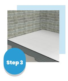
Lay tiles after curing (minimum tile dimension are 100 x 100 mm with thickness not less than 7 mm).
