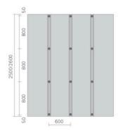
Use 600 mm wide MARMOX BOARD with min. 20 mm thickness for stud frame distance of 600 mm.
