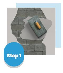
Clean surface underneath the boards, remove and replace loose plaster. Level cavities if required.
