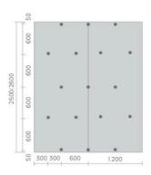
Positioning of dowels for full surface bonding of boards with 1200 mm width starting with 10 mm thickness.
