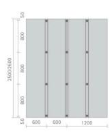
Stud frame distance of 600 mm is recommended for 1200 mm wide MARMOX BOARD with minimum 20 mm thickness.
