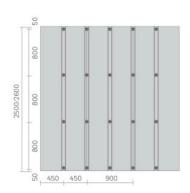
Stud frame distance of 450 mm is recommended for 900 mm wide MARMOX BOARD with 10 mm and 12.5 mm thickness.
