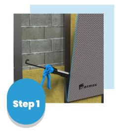
Screw the MARMOX BOARD to the timber or metal frame tightly by using MARMOX washers along with drywall screws. Seal wet areas joints and cover all washers with MS Polymer.
