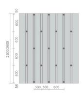
600 mm wide MARMOX BOARD with 10 mm and 12.5 mm thickness can be used if stud frame distance is 300 mm.
