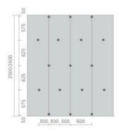
Positioning of dowels for full surface bonding of boards starting with 4 mm thickness.
