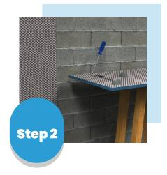
Punch holes (5 per m² for ceramic tiles + 8 per m² for natural stone) into the MARMOX BOARD by using a screwdriver then apply over the holes with a dab of flexible tile adhesive.
