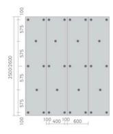
Positioning of dowels on uneven or rough wall surface with dab of flexible tile adhesive with min 20 mm thickness.
